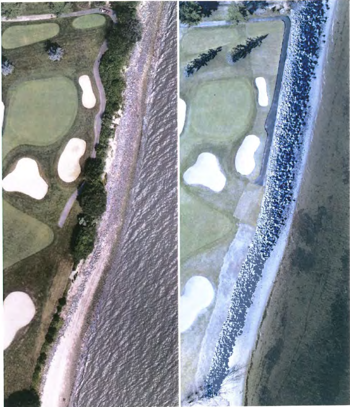
Aerial imagery comparison showing coastal vegetation, habitat, and shoreline access destroyed or lost by construction of illegal wall. Left image from Summer 2022, Right image from Spring 2023.
